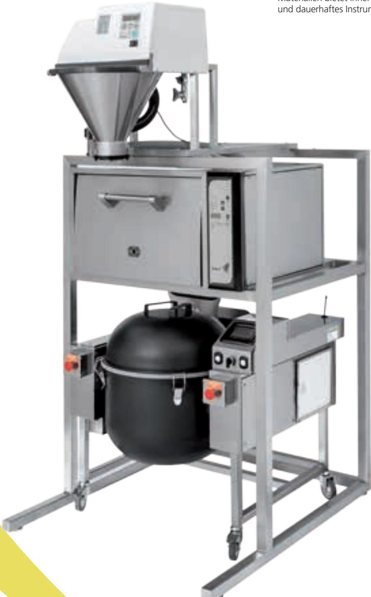
**EN** TORA incorporates the entire sushi rice preparation cycle into a single solution. It is made up of a complete stainless steel 304 column which perfectly holds the rice washing machine, the oven and the mixer. An ideal and extremely compact solution for all activities within ethnic restaurants which need to rationally organise the available space. The manufacturing robustness and the quality of materials make it an extremely reliable tool which is able to withstand time.
