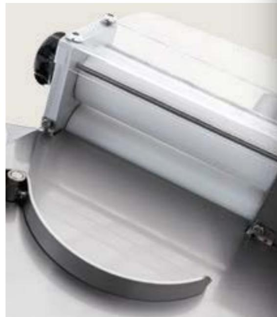
Touch & Go function ensures optimal results and high production volumes. Its unique feature is the automatic start-up of the rollers via sensors.
