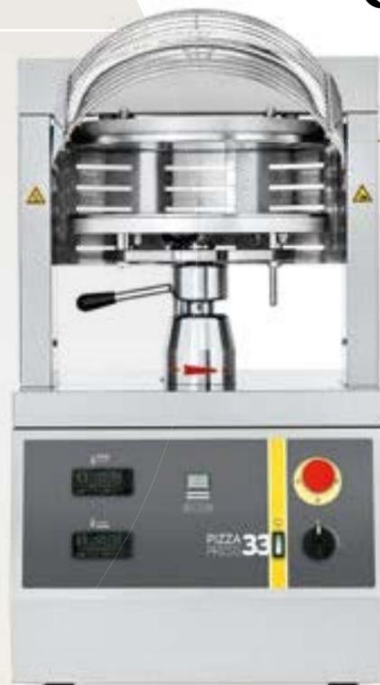
**✓** The metal wire safety grid offers the maximum protection
