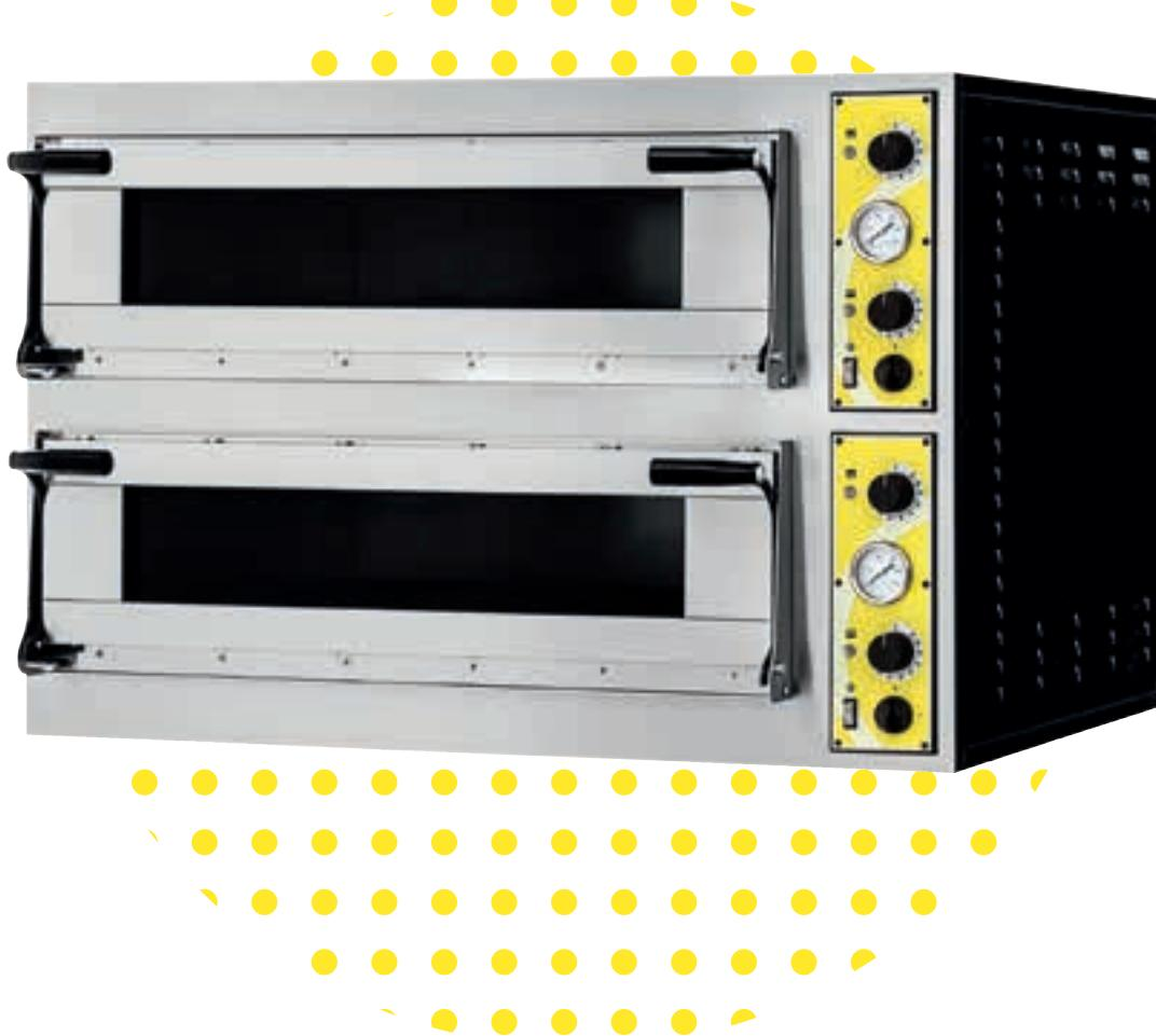
The electric oven is made of stainless steel and prepainted steel, it is equipped with: cooking surface in refractory stones, sheathed heating elements, internal lighting and rock wool insulation. The standard power supply is 400V three-phases + neutral. Special voltages are available on request.
