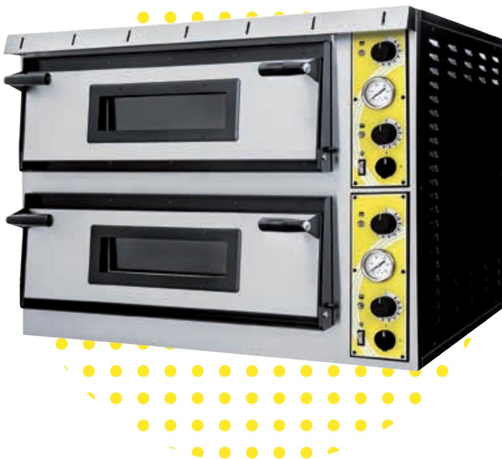
The electric oven is made of stainless steel and prepainted steel and it is equipped with: cooking surface in refractory stones, 3 sheathed heating elements on the top and 3 on the bottom, removable glass door for a better cleaning, internal lighting, rock wool insulation. The design is enriched by a little hood, which makes the oven elegant. The standard power supply is 400V three phases + neutral. Special voltages are available on request.
