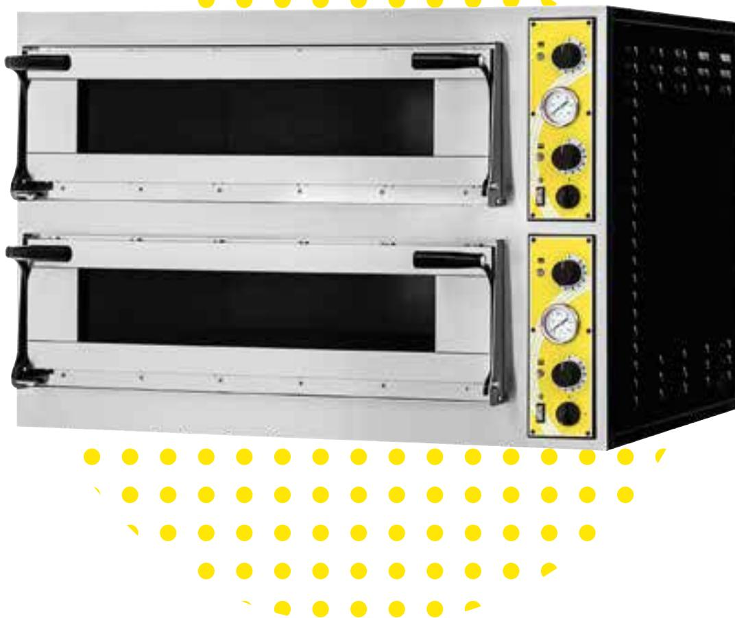
The electric oven is made of stainless steel and prepainted steel, it is equipped with: cooking surface in refractory stones, sheathed heating elements, internal lighting and rock wool insulation. The standard power supply is 400V three-phases + neutral. Special voltages are available on request.
