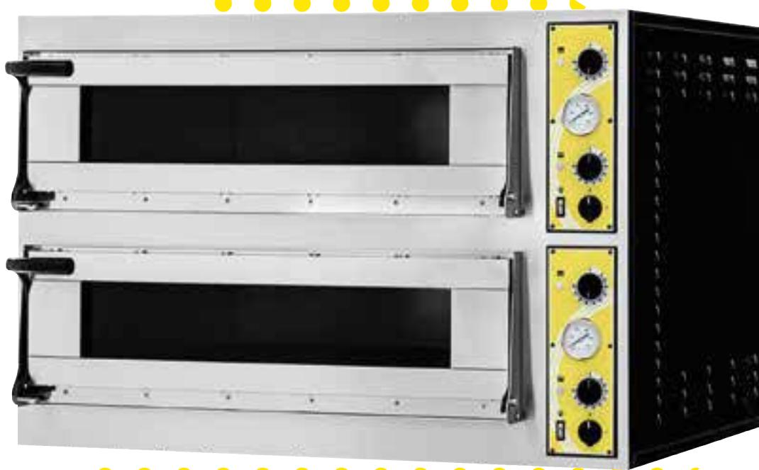
The electric oven is made of stainless steel and prepainted steel, it is equipped with: cooking surface in refractory stones, sheathed heating elements, internal lighting and rock wool insulation. The standard power supply is 400V three-phases + neutral. Special voltages are available on request.
